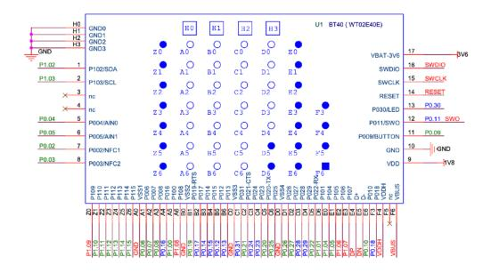
WT02C40C production version pin assignments. Pins 17, 18, 19, and 20 are antenna connection for WT02P40P only.
