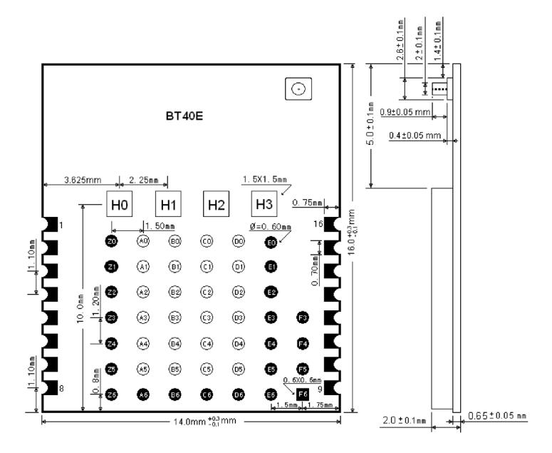
The following is BT40N mechanical drawings.
