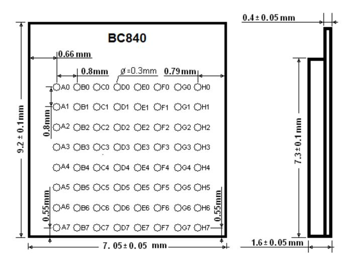
BC840M mechanical drawings, top view.
