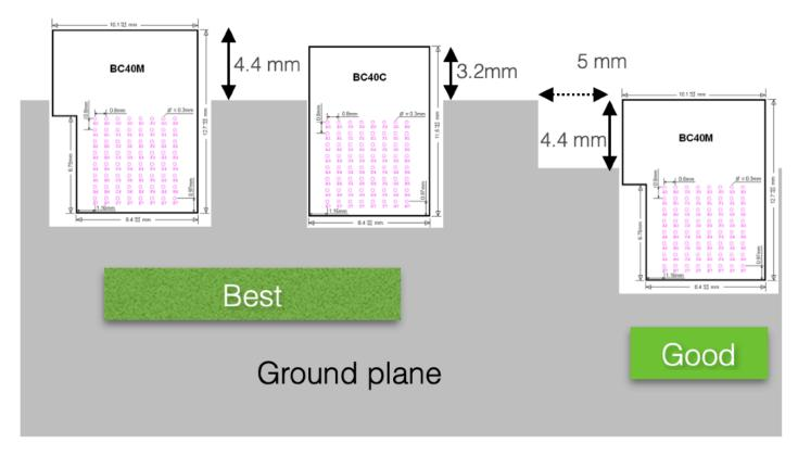
The following figure shows recommended mounting of BC40C module on the host PCB.
