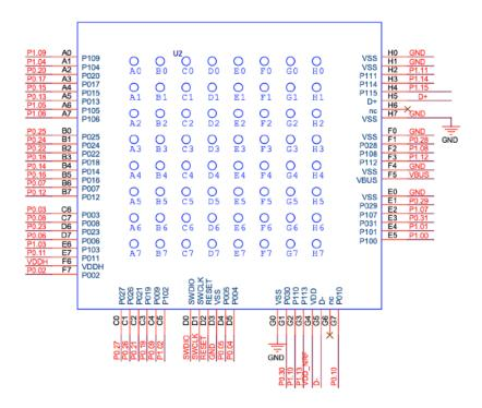
BC40P pin assignment is below. It has two additional pins for external antenna connection.
