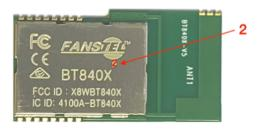
BT840X-p and BT840XE-p: All BT840X-p and BT840XE-p are new version devices. There is a "P" marking above the "X" or "XE" to indicate supporting of approtect.
