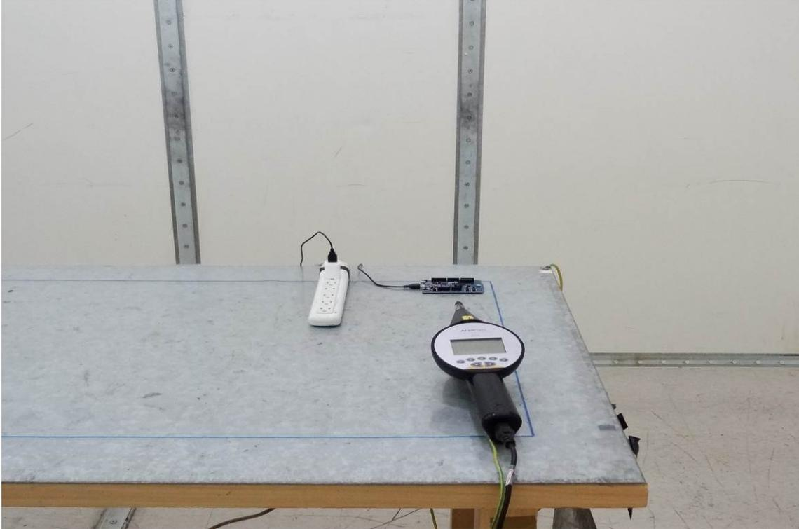
**RADIATED ELECTROMAGNETIC FIELD (EN 61000-4-3)**
