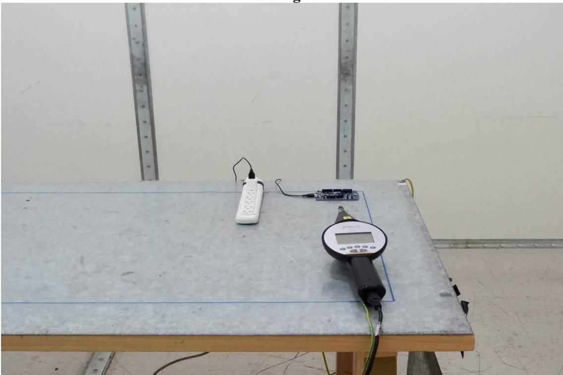
**ELECTROSTATIC DISCHARGE TEST (EN 61000-4-2)**
