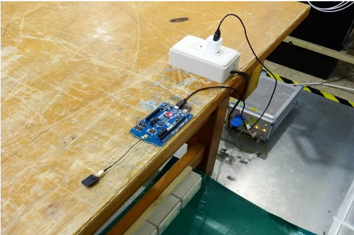
**ELECTROSTATIC DISCHARGE TEST (EN 61000-4-2)**
