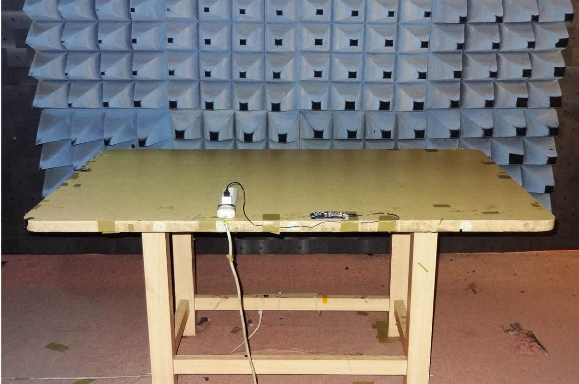
**RADIATED ELECTROMAGNETIC FIELD (EN 61000-4-3)**
